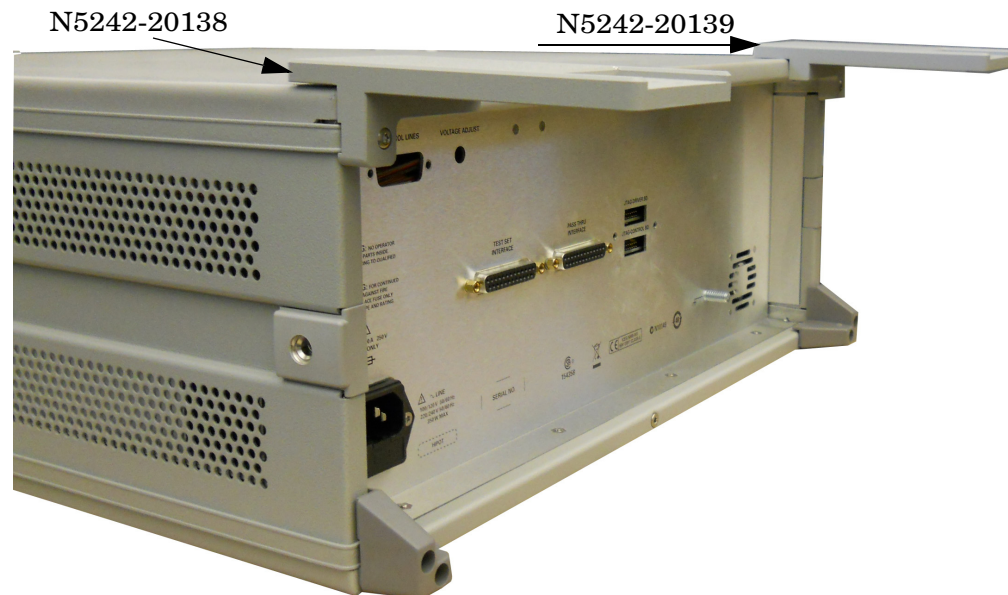
Figure 7 Install Locking Feet on Test Set
