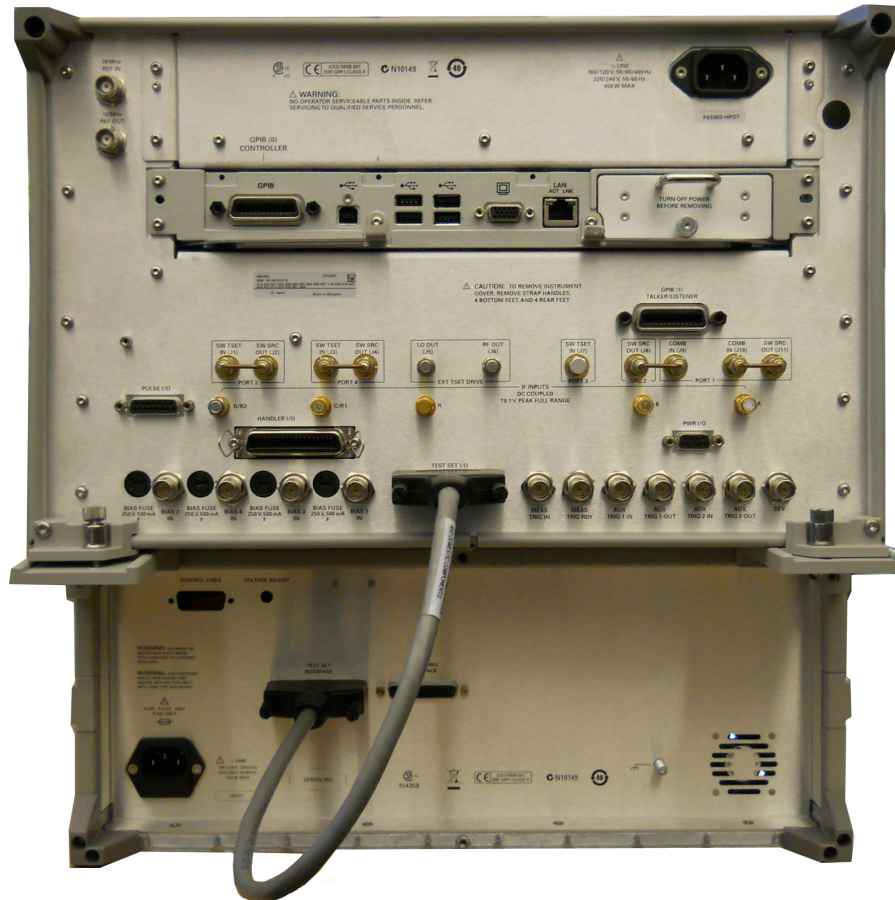
Figure 11 Rear Panel N5245A with U3045AM08
