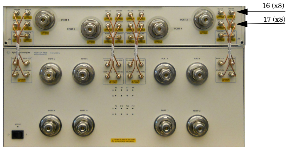
Figure 10 PNA-X RF Interface Cable Connections
